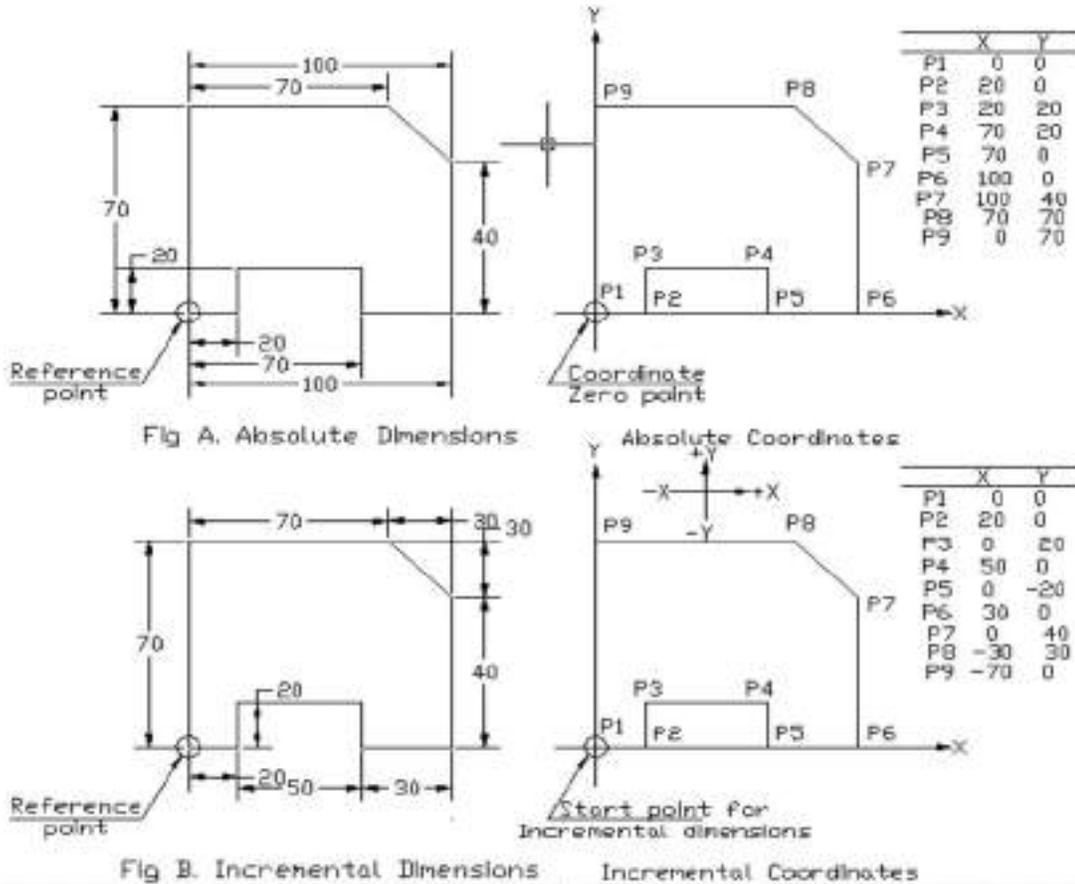
**1. Absolute Dimension System:** Data in absolute dimension system always refer to a fixed reference point in the drawing as shown in figure A above. This point has the function of a coordinate zero point as in figure B. The dimension lines run parallel to the coordinate axes and always start at the reference point. Absolute dimensions are also called as “Reference dimensions”.
