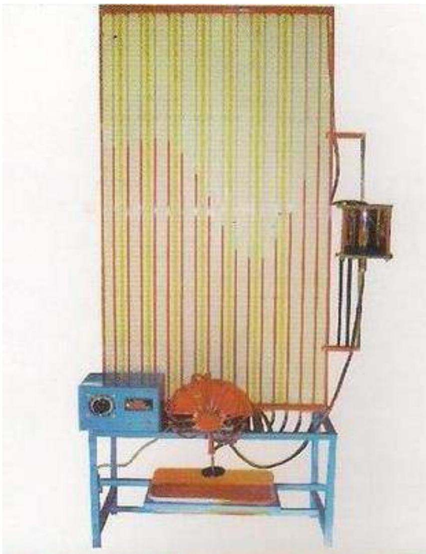
Figure 8: Journal Bearing Apparatus
